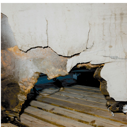
Recovered right solid rocket booster showing the hole caused by the plume.
